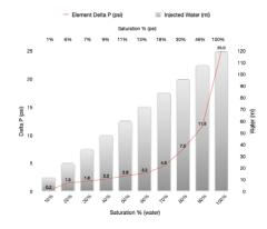
Water and emulsions cause up to 15% of power loss, thus up to 15% increase in fuel consumption. All ISO 4406 contamination control plans must contemplate water and emulsions with SAE J1488 certified systems.
