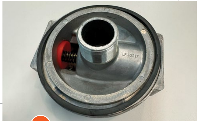
INCORRECTLY INSTALLED O-RING
