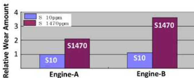
Figure DF - 10: Relative Cylinder Bore Wear in Endurance Test with High and Low Sulphur Fuels
