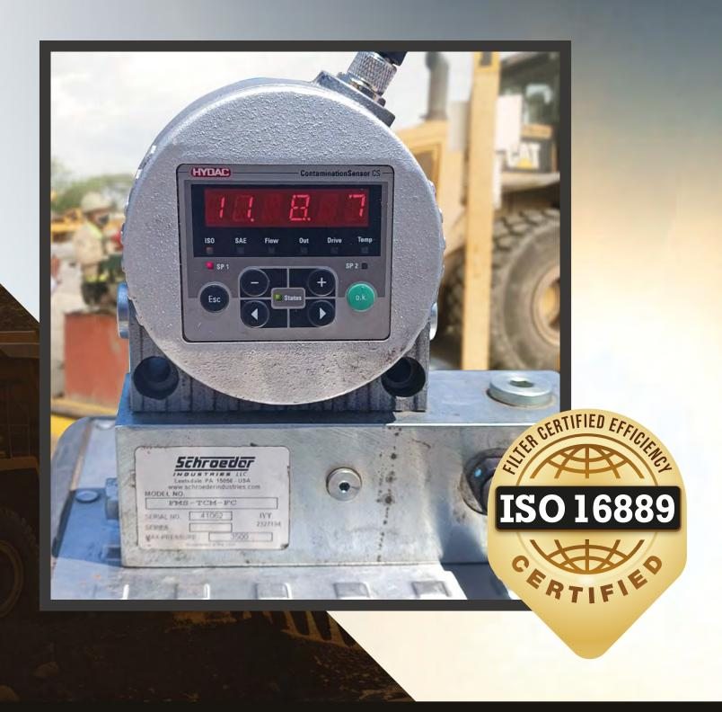
Since 2017, Agrenic has implemented FMS filtration, successfully maintaining certified diesel below code 11/8/7, with effective control of water and emulsions. We have seen several benefits, including cleaner combustion, protection of injection systems, and a reduction in pollutant emissions—contributing to environmental protection."
